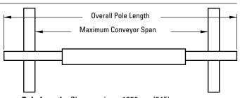
Pole Length Cleaner size + 1350mm (54") Maximum Conveyor Span Cleaner size + 1100mm (44")
